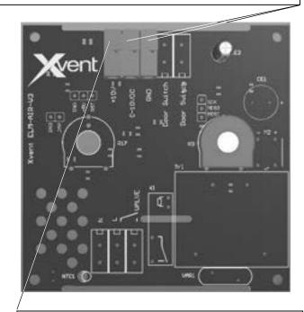
**Terminal clamp for regulator power supply** clamp +10V intended for regulator power supply Max. current capacity of regulator: 10mA *Recommended cross-section of conductors:* from 0.5 mm<sup>2</sup>to 1.5mm<sup>2</sup>.
