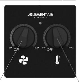
Continuous fan speed regulator allows continuous fan speed adjustment in any position from minimum to maximum speed as required by the user. The "OFF" position allows the entire regulator to be switched off. The "OFF" position does not ensure isolation of the controlled equipment from the supply voltage; isolation needs to be ensured separately on the supply side.
