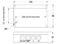
Always install the HUB on a solid surface to prevent it from being accidentally released and consequently damaged.
