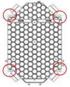
b) Choose the installation position taking into account the location of the condensate outlet. Align the anchor holes according to the dimensions on the unit, drill and mount the unit leveled using suitable screws. Do not tilt the unit.
