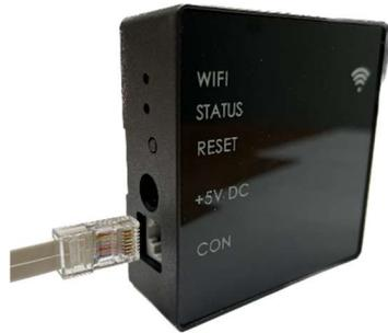
**3** Connect the converter power supply connector into the converter (+5V DC) and the adapter to the electrical mains (230V)
