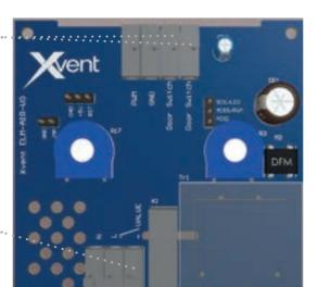
For maximum use of featuresThe Elementair-E has contacts labeled "Door Switch" and "Valve".
