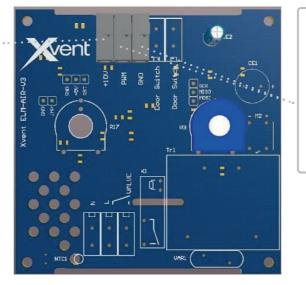
Terminals for connection of EC fan Description: terminals for connection of control voltage from EC fan PWM / 0-10VDC (+); GND with a resistance of  $10k\Omega$ . Control range 2-10VDC max 0,3mA
