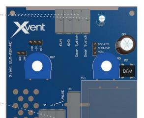
For maximum use of featuresThe Elementair-E has contacts labeled "Door Switch" and "Valve".
