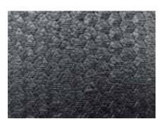
Body of the unit is made from black **EPP**. (expanded polypropylene).
